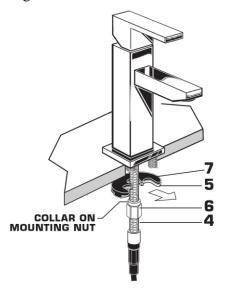
From below, push GASKET [7] and RETAINING WASHER [5] onto MOUNTING STUD [4]. Secure Faucet with MOUNTING NUT [6], pulling faucet to front of sink, so SUPPLIES [3] rests against mounting hole. Before final tightening, make sure collar on MOUNTING NUT [6] is seated into RETAINING WASHER [5].
