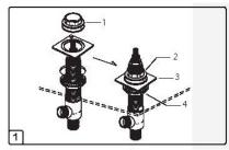
Install Valve bodies (MAKE SURE the main water supply is completely turned off):
